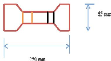
d) Dog bone specimen for tensile test;
