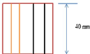
a) Cube specimen for compression test
