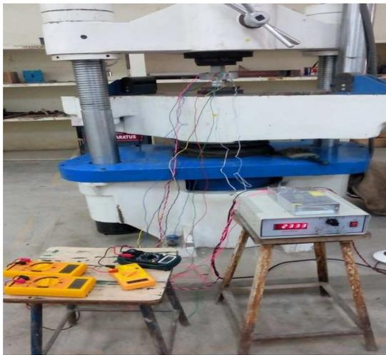
Fig. 3. Compression test setup for joint Specimen.
