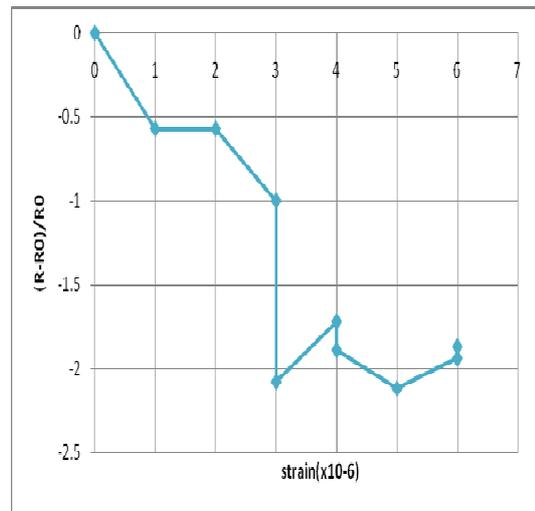
Graph 4 Test result graph of Dog-bone specimen with normal mix + Latex + fiber
